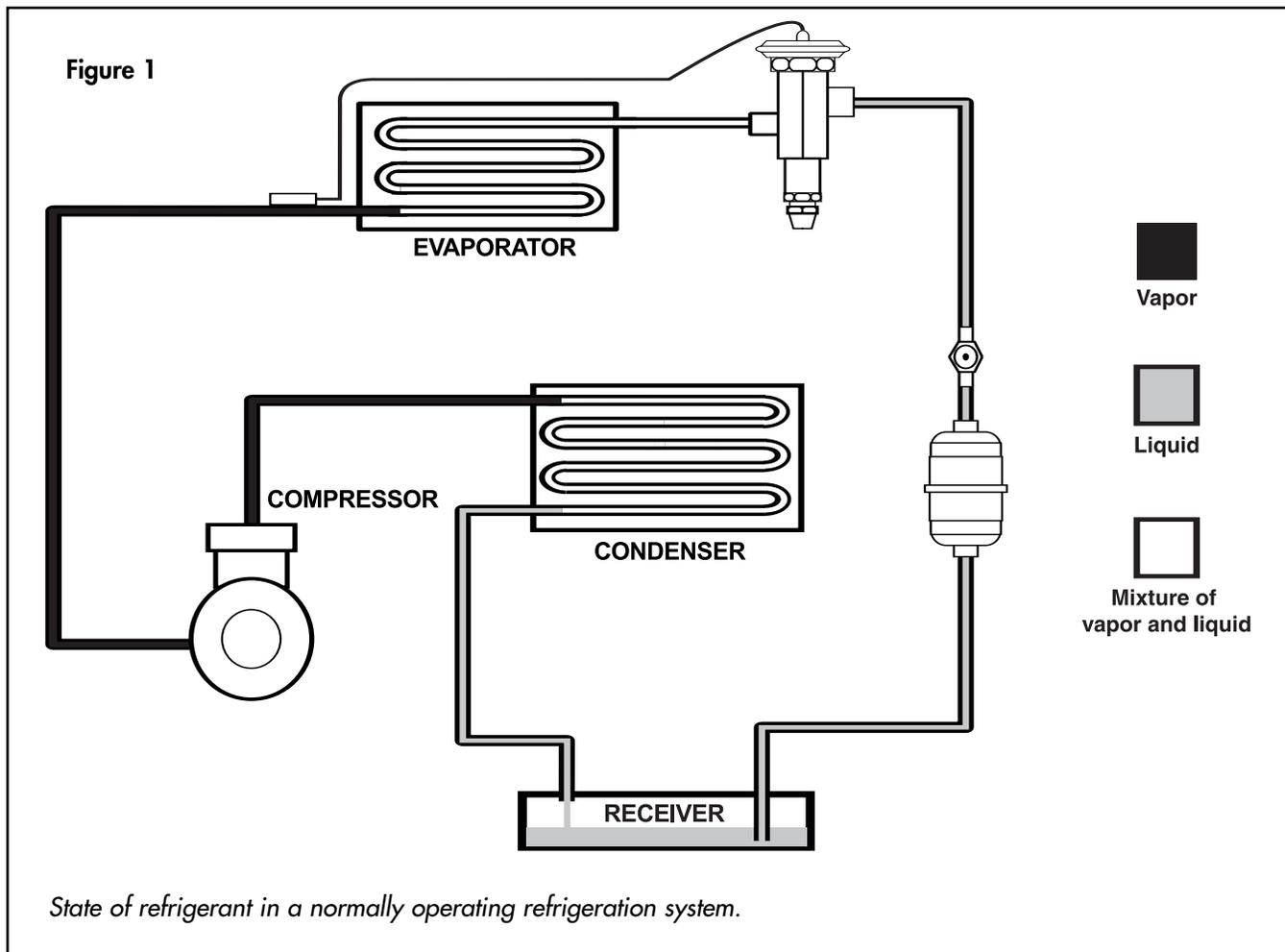
**Figure 1** illustrates the form in which refrigerant is found at various points in a normal operating refrigeration system.
