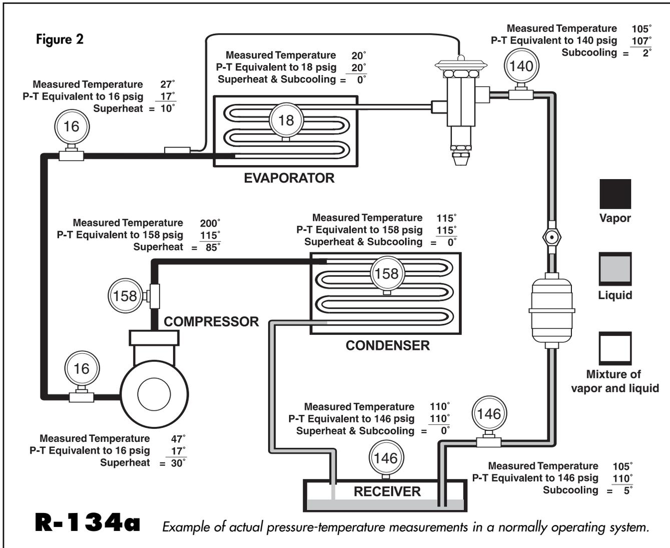
temperature and saturation temperature), it is determined that the superheat is 85°F.
