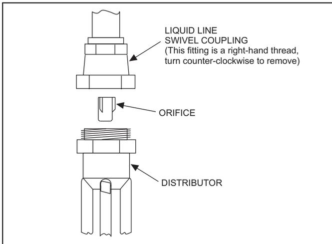
FIGURE 5: Orifice Installation
