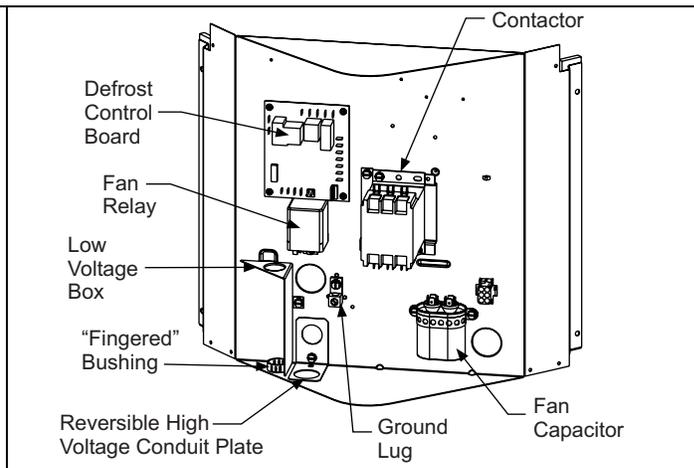
FIGURE 7: Outdoor Unit Control Box - Three Phase
