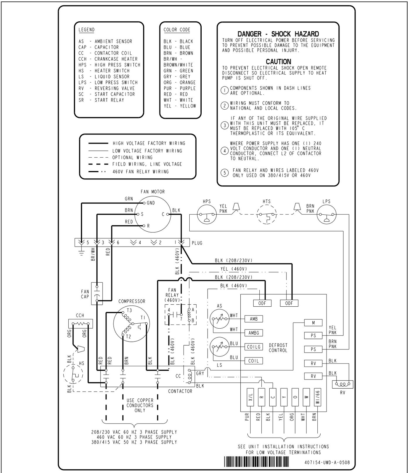
FIGURE 16: Wiring Diagram - Three Phase (Demand Defrost)
