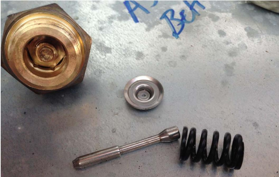
We used a clean rag lightly dipped in SUPCO 88 to clean the valve body by wiping it down. The following two pictures show the valve body before and after:
