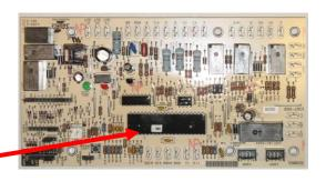
For units manufactured before September 2009, a labor allowance of 90 minutes will be provided for replacement of the previous version of York Guard VI control (080) to remedy incomplete defrost issues. The Source One part number for the new board is \$1-33102957000.
